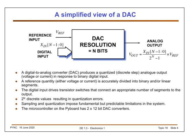
A **digital-to-analog converter** produces an analogue output which corresponds to the value of the digital input signal. The analogue output value corresponds to the relative value of the digital input signal with respect to a fixed reference value V<sub>REF</sub> and, in its most basic form, is determined by the relationship above.
