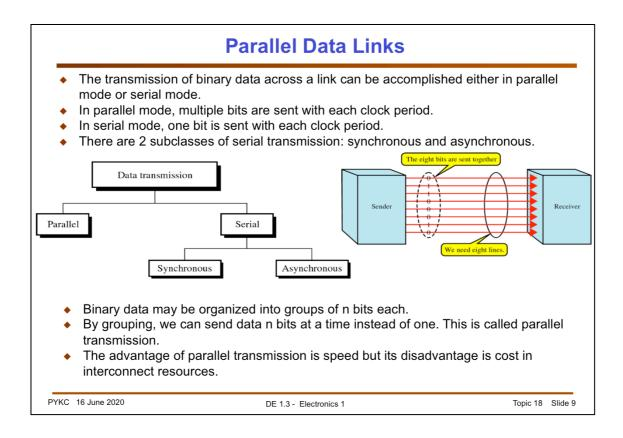
Transferring data between two devices or modules can be done in two main methods: parallel and serial. In parallel transmission, a data word (which has n bits) are send together all at once. The advantage is speed of transfer. Example of this is the memory interface with microprocessor. The disadvantage is that you need n wires, which could be costly. For example, pins on the packaging of a chip is expensive.
