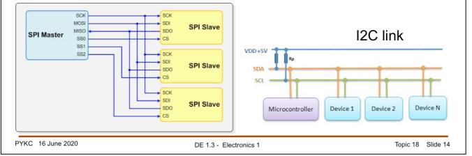
Two of the most common synchronous serial links used in industry are: I2C (Inter-Integrated Circuit) and SPI (serial peripheral interface).
