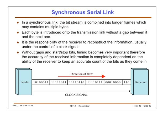
Asynchronous serial transmission is only suitable for low data rate link between modules. For higher speed communication between two modules on the same chip or on the same PCB, a synchronous serial link is much better. The transfer of data in a synchronous serial link requires the use of a clock signal from one module to another module. The module that produces the clock signal is known as the **master** device. The other module is known as the **slave device**.
