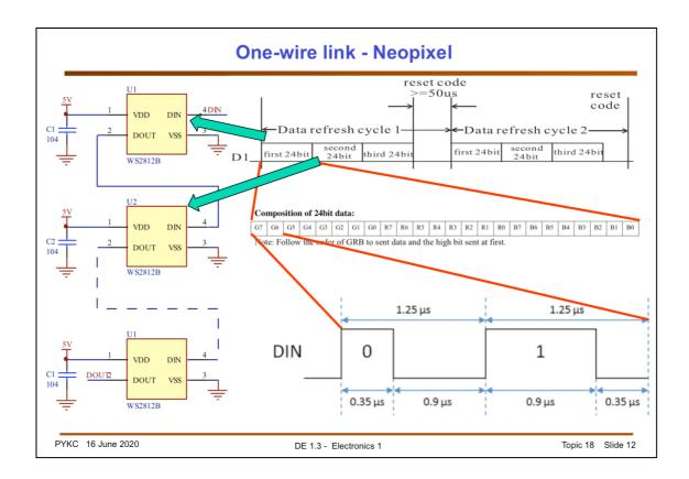
Neopixel is another example of asynchronise link that uses only one data wire. Neopixel is actually a fancy name for the WS2812B three colour LED. The Neopixel strip you received in the Home Lab Kit has 8 LEDs connected in series (called daisy-chain) as shown in the slide. Each LED module contains three separate LEDs: R, G and B.
