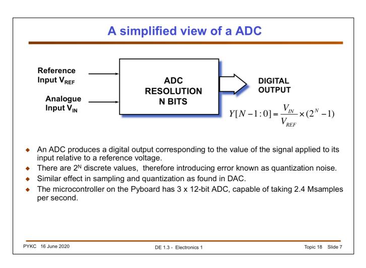
An analogue-to-digital converter produces a digital output which corresponds to the value of the analogue input signal. The digital output value corresponds to the relative value of the analogue input signal with respect to a fixed reference voltage and, in its most basic form, is determined by the relationship above.
