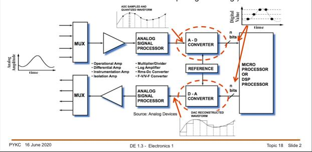
The real world problem consists of taking a continuous signal (analog) and applying decisions by means of digital signal processing to the signal. DSP allows for efficient and cost effective means of allocating information (bandwidth, capacity) correctly.
