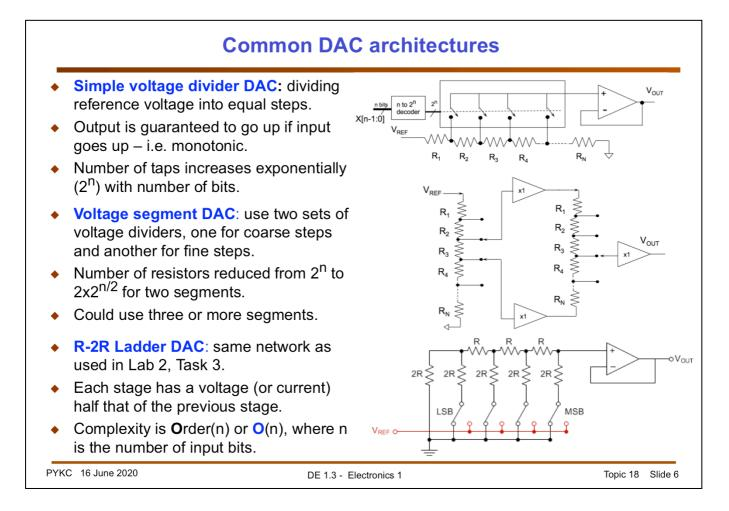
The simplest DAC circuit is that of a **voltage or potential divider**. Here all resistors are identical and  $V_{REF}$  is simply divided into N equal steps. This architecture is also known as **a String DAC** (having a string of identical resistors). The complexity grows exponentially with number of input data bits. We call this of Order(2<sup>n</sup>).
