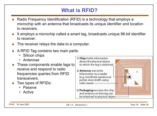
A Radio-Frequency IDentification system has three parts:
