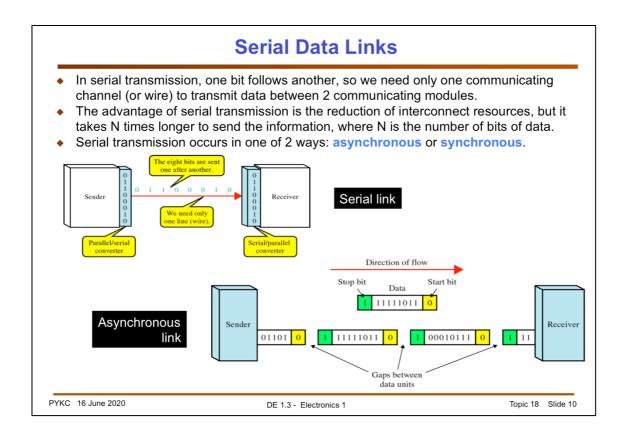
In serial transmission, one bit follows another, so we need only one communicating channel (or wire) to transmit data between 2 communicating modules. The advantage of serial transmission is the reduction of interconnect resources, but it takes N times longer to send the information, where N is the number of bits of data.
